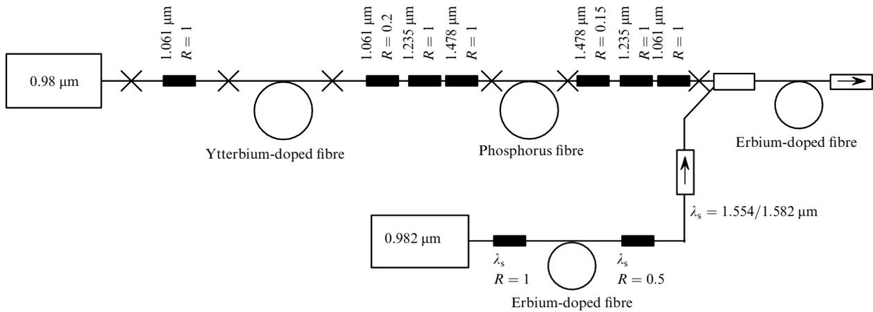
**Figure 1.** Scheme of the setup (splicings are shown by crosses, and the dark rectangles correspond to gratings).
