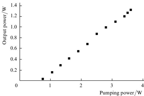
**Figure 2.** Dependence of the output power of a Raman converter at 1478 nm on the pumping power of the ytterbium laser.
