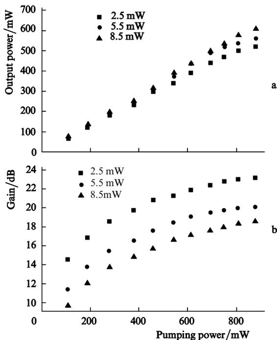
Figure 4. Dependences of the output power (a) and the gain (b) of an erbium-doped fibre amplifier at 1582 nm on the pumping power at 1478 nm.
