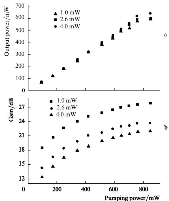
**Figure 3.** Dependences of the output power (a) and the gain (b) of an erbium-doped fibre amplifier at 1554 nm on the pumping power at 1478 nm.
