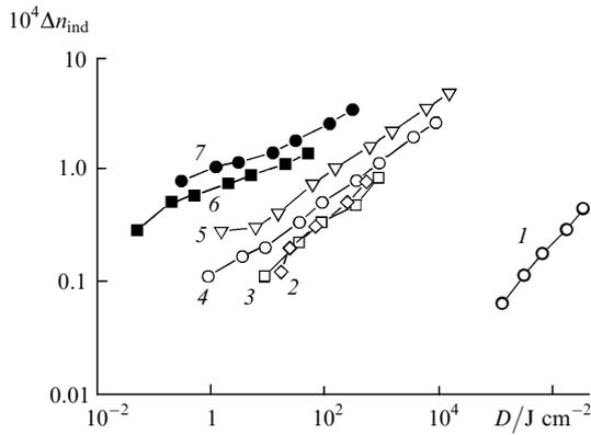
**Figure 3.** Dependences of the induced RI on the dose of cw  $\lambda = 333\text{--}364$  nm radiation of  $300\text{ W cm}^{-2}$  intensity (1) and of cw  $\lambda = 244$  nm radiation of intensities  $0.08\text{ W cm}^{-2}$  (2),  $0.86\text{ W cm}^{-2}$  (3),  $8.8\text{ W cm}^{-2}$  (4), and  $15\text{ W cm}^{-2}$  (5), and also of pulsed  $\lambda = 248$  nm radiation of energy densities  $50\text{ mJ cm}^{-2}$  (6) and  $300\text{ mJ cm}^{-2}$  (7).
