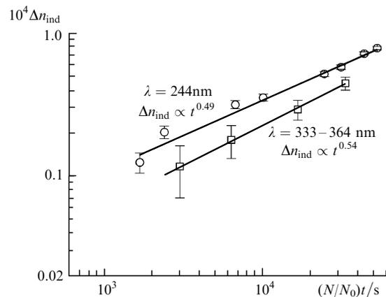
**Figure 4.** Dependences of  $\Delta n_{\text{ind}}$  on  $(N/N_0)t$  for irradiation at  $\lambda = 244$  and  $333\text{--}364$  nm.
