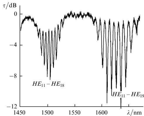
Figure 1. Transmission spectrum of a Mach-Zehnder interferometer.
