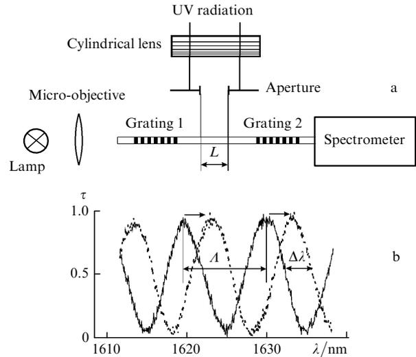
Figure 2. System used to study the dynamics of the RI changes induced in the core of a fibre waveguide (a) and the changes in the transmission spectrum of an interferometer as a result of UV irradiation (b).
