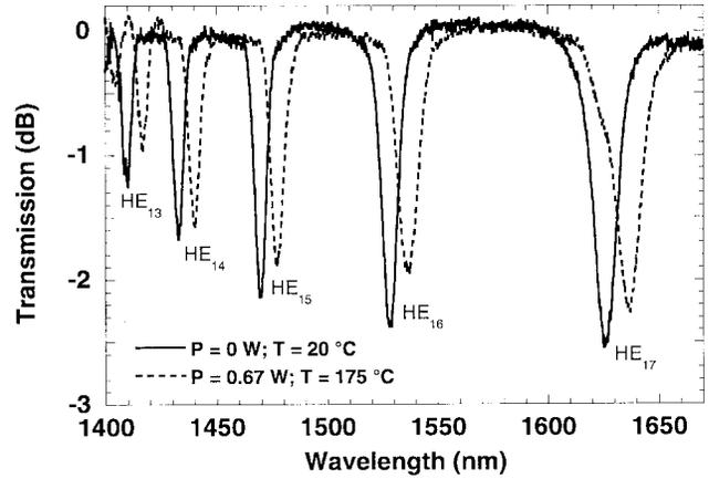
Fig. 2. Transmission spectra of the LPG at room temperature without electrical heating (solid curve) and for an applied power of 0.67 W (dashed curve).
