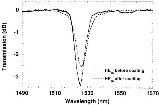
Fig. 1. LPG transmission spectra for HE<sub>16</sub> mode coupling before (solid curve) and after (dashed curve) the deposition of the thin-film metal coating.
