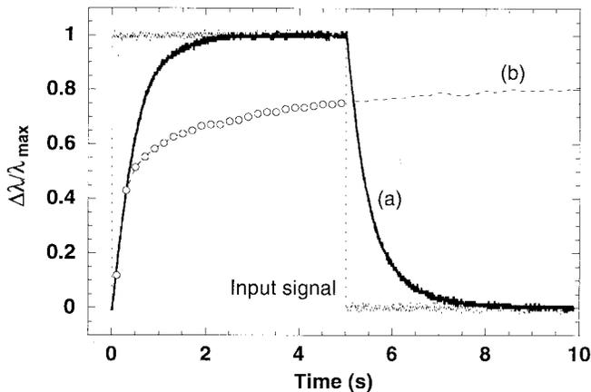
Fig. 4. Response of the tunable filter to a rectangular electrical signal. (a) Fiber surrounded by air. (b) Fiber placed on Teflon substrate.
