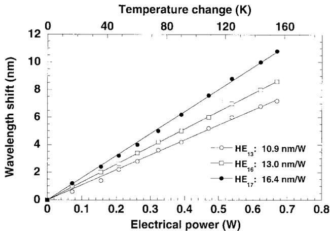
Fig. 3. Dependence of the wavelength shift of resonance peaks on the applied electrical power.
