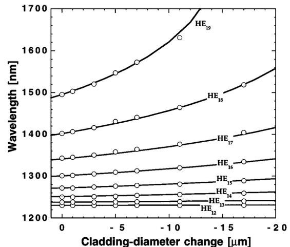
Fig. 3. Experimental (circles) and theoretical (curves) resonance wavelengths' positions as a function of cladding-diameter change.
