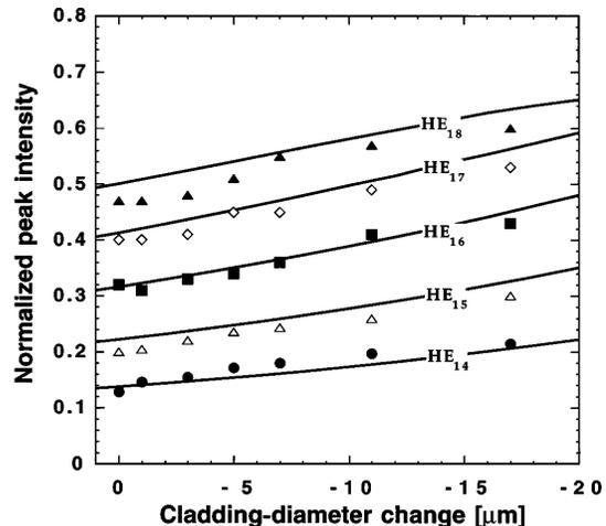
Fig. 4. Experimental (symbols) and theoretical (curves) normalized peaks' intensities as a function of cladding-diameter changes.
