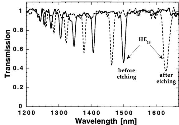
Fig. 2. Initial spectrum (solid curve) and the spectrum after 5 min of HF etching (dashed curve) for a long-period grating (see grating parameters in text).
