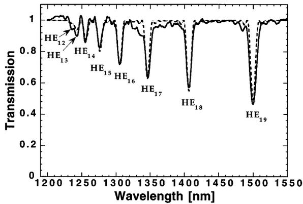
Fig. 1. Experimental (solid curve) and theoretical (dashed curve) transmission spectra of a long-period grating with 17-mm length ( $\Lambda = 200 \mu\text{m}$ ).
