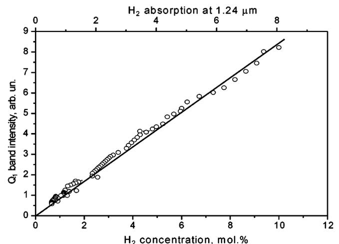
Fig. 7. Dependence of integral intensity of Raman  $Q_1$  band on hydrogen concentration in the fiber and/or absorption band intensity at 1.24  $\mu\text{m}$ .
