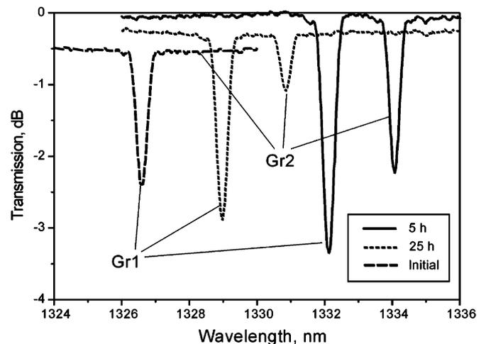
Fig. 5. Transmission spectra of Bragg gratings measured before hydrogen loading, as well as in 5 and 25 h after the loading was over. For better recognition the spectra were displaced by 0.25 dB relatively to each other.
