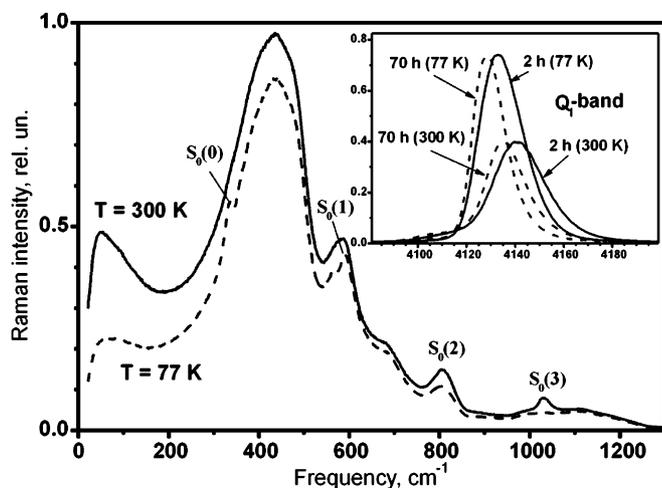
Fig. 2. Raman spectra of H<sub>2</sub> loaded fiber number 1 measured at 77 K (dotted curve) and 300 K (solid curve). The Q<sub>1</sub> band spectra of H<sub>2</sub> molecules in this fiber measured in 2 h (solid curves) and 70 h (dotted curves) after hydrogen treatment are shown in the inset. For better presentation the spectra in the inset are normalized in pairs to the band peak intensity.
