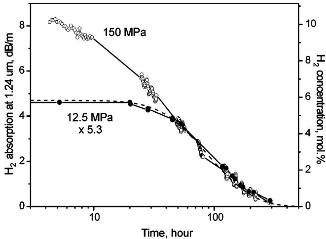
Fig. 4. Time dependence of the 1.24  $\mu\text{m}$  band intensity (open circles) during hydrogen out-diffusion from fiber number 4 (150 MPa). Full circles show the same dependence at a loading pressure of 12.5 MPa (for better comparison at large times the absorption coefficient is multiplied by a factor of 5.3). Dotted curve represents the results of calculation of hydrogen escape performed with a constant diffusion coefficient.
