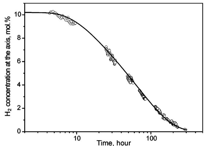
Fig. 8. Concentration of molecular hydrogen at the fiber axis measured (experimental points) and calculated with taking barodiffusion into consideration (solid curve).
