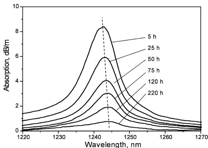
Fig. 3. Absorption spectra of molecular hydrogen near 1.24 μm measured in optical fiber number 4 for different time intervals after hydrogen loading at 170 MPa.
