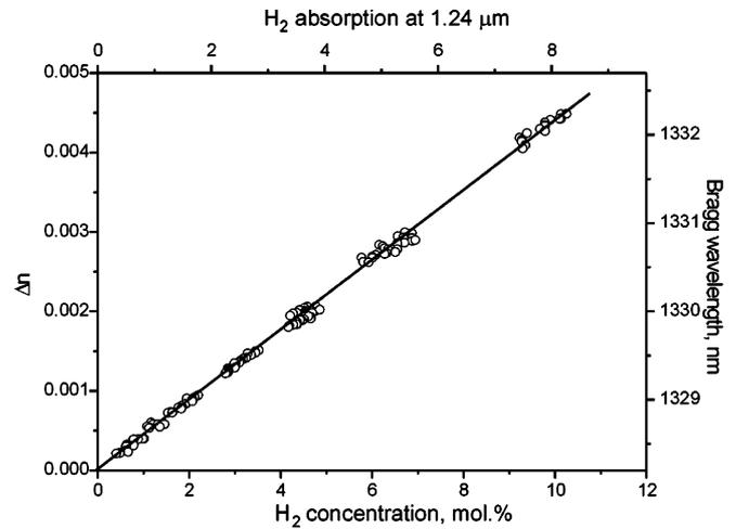
Fig. 6. Dependence of hydrogen-induced mean index change on hydrogen concentration in the glass network.
