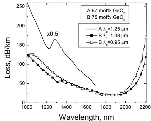
Fig. 2. Optical loss spectra in SMFs A and B
