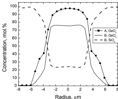
Fig. 1. GeO<sub>2</sub> and SiO<sub>2</sub> concentration profiles measured in MM fibres A and B by X-ray microanalysis
