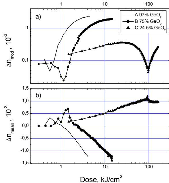
Fig.3. Index modulation  $\Delta n_{\text{mod}}$  (a) and of mean index change  $\Delta n_{\text{mean}}$  (b) in the Bragg gratings written in fibres A, B and C vs dose of 244-nm radiation.
