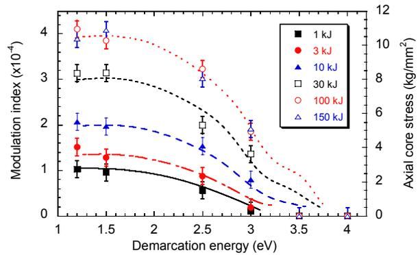
Fig. 6: Correlation of index modulation and UV-induced axial core stress changes for six different total doses.
