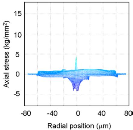
*Fig. 1: Axial two-dimensional stress profile of the pristine fiber.*
