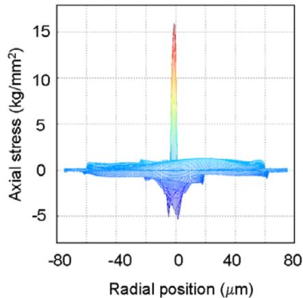
*Fig. 2: Axial core stress increase after irradiation with a total dose of  $150 \text{ kJ/cm}^2$ .*
