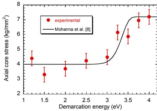
Fig. 5: Residual axial core stress as a function of demarcation energy for the pristine fiber.
